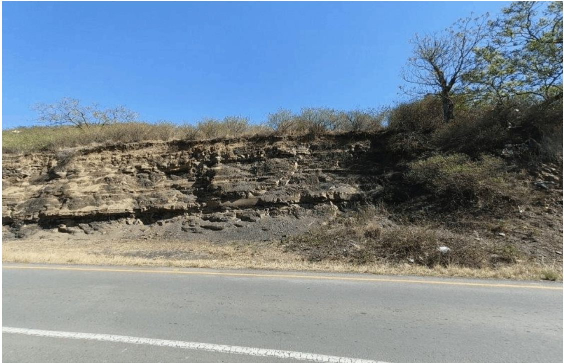
Figure 5 - Moderately Weathered Shale
